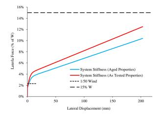
Figure 4. Force displacement properties of LRBs – As-Tested and Aged Properties.
