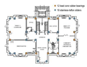
Figure 6. Basement plan showing locations of bearings and sliders.
