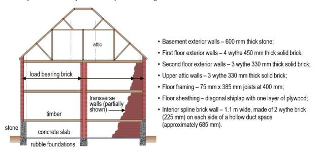
Figure 1. Cross section of original structure and description of elements.
